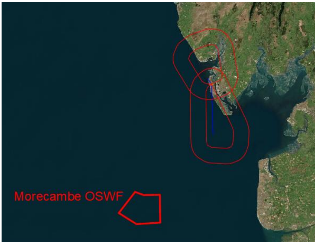
Figure 173 – Windfarm vs ILS/DME RWY 35 Alternative Baseturn Reversals
