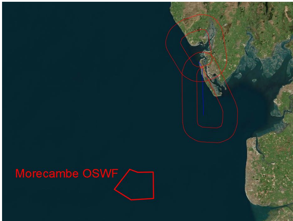
Figure 181 - Windfarm vs NDB(L)/DME RWY 35 Alternative Base Turn Reversals
