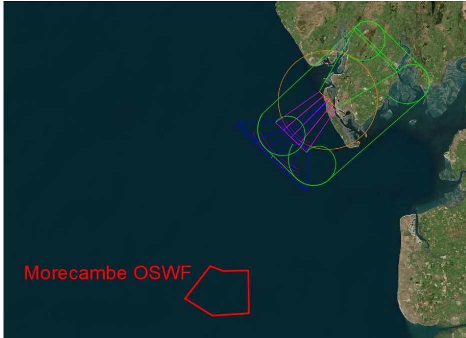
Figure 183 – Windfarm vs NDB(L)/DME to Aerodrome
