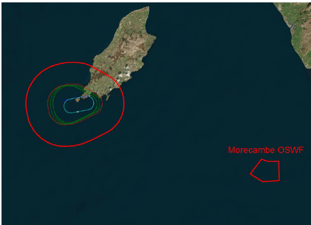
Figure 109 - Windfarm vs VOR/DME RWY 08 Extended Holding
